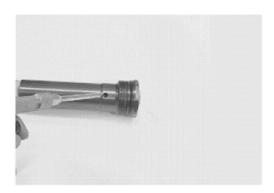
• With the damper rod in horizontal position, move the inner rod by hand to inspect it if operating smoothly.
