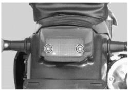
• Remove the brake light/taillight bulb.
