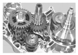
Install the gearshift fork shafts.
