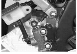
Loosen the locknut ① and remove the master cylinder assembly.
