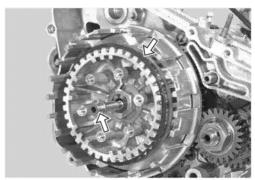
• Flatten the clutch sleeve hub washer.
