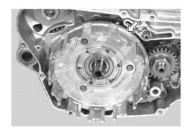
• Remove the cam chain tensioner ① and cam chain ②.
