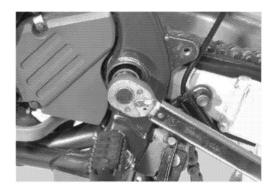
• Tighten the cushion lever mounting nut to the specified torque.
