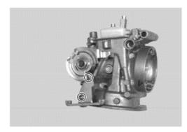
• Remove the float pin (10), float (11), and needle valve (12).
