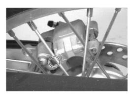
• Tighten the brake pad mounting pin to the specified torque.
