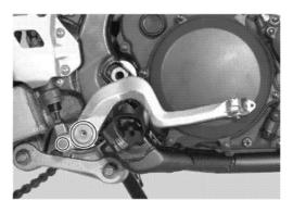
• Disconnect the horn coupler ① and remove the horn ②.
