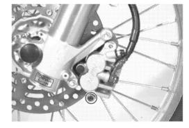
· Remove the brake pads.
