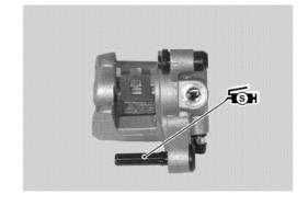
• Tighten the brake hose union bolt to the specified torque.
