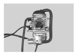
• Remove the piston valve control solenoid ① and joint pipe ② (Except for E-03, 28, 33).
