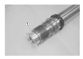
Insert the inner tube into the outer tube and install the oil seal using the special tool.
