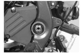
• Remove the chain buffer ③ and brake hose guides ④.
