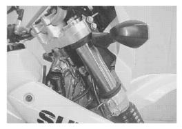
Tighten the boot clamp screws with the boots touching to the steering stem.
