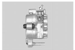
Place a rag over the brake caliper pistons to prevent them from popping out, and then force out the pistons using compressed air.
