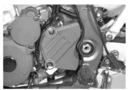
• Flatten the washer ① and remove the engine sprocket nut ② while pressing down on the rear brake pedal.
