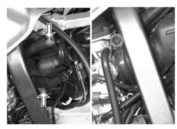
· Remove the overflow tank mounting bolt.
