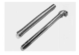
• Measure the inner tube runout using the V-blocks and dial gauge.
