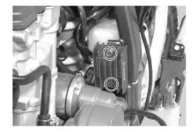
• Remove the engine coolant overflow tank mounting bolt.
