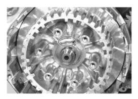
• Hold the clutch sleeve hub using the special tool, and then remove the clutch sleeve hub nut.
