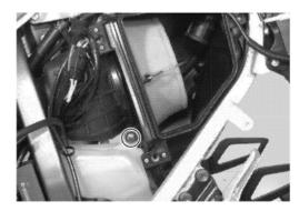
Remove the seat rail with air cleaner case assembly.
