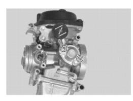
• Remove the starter plunger assembly.
