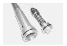
With the damper rod in fully extended position, pour the specified amount of fork oil.
