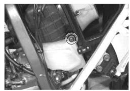
• Disconnect the spark plug cap ①, engine oil breather hose ②, engine oil hose ③, and remove the engine oil tank ④.
