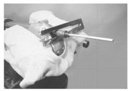
• With the outer tube compressed by hands, remove the special tool.
