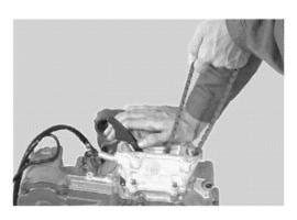
\* There is a holder for the bottom end of the cam chain guide cast in the crankcase. Make sure that the guide ③ is inserted properly or binding of the cam chain and guide may result.
