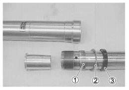
• Install the oil lock piece 1 into the inne tube.
