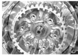
Install the spring washer seat ① and spring washer ② onto the clutch sleeve hub correctly.
