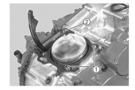
Hold each piston ring with the piston ring sections positioned correctly and put it into the cylinder. Make sure that the piston rings are caught by the cylinder skirt.
