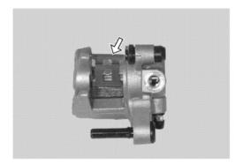
Place a rag over the brake caliper piston to prevent them from popping out and then force out the piston using compressed air.
