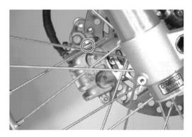
• Tighten the brake pad mounting pin to the specified torque.
