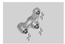
Remove the cushion lever needle bearings using the special tools.
