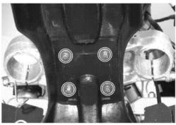
• Remove the handlebar 1) and ignition switch 2).
