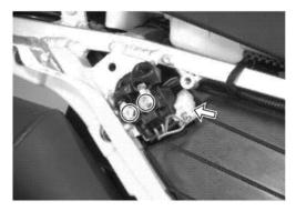
Apply 12 V to the terminals and check for continuity between the positive and negative terminals using the multi circuit tester. If the starter relay clicks and continuity is found, the relay is ok.
