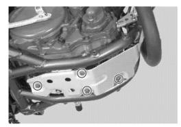
• Remove the CDI unit cover ① and disconnect the neutral switch coupler ②.
