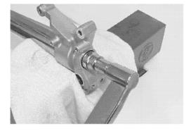
• Loosen and remove the fork cap bolt (sub-tank) from the outer tube and slowly slide down the outer tube.
