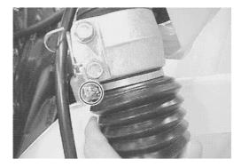
• Fix the boot to the boot holder with a new clamp.
