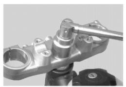
Remove the washer ③ and steering stem upper bracket ④.
