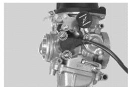
• Remove the coasting richer pump assembly.
